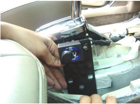
9. Position the lock with the pin behind the gearshift. And remove the carpet of the front seat and check the position of the bracket.
