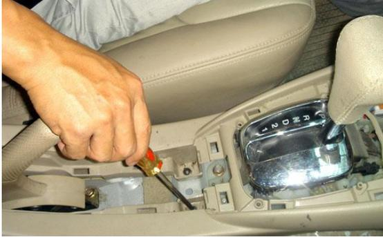
5. Lose the inside screws of gearbox.
