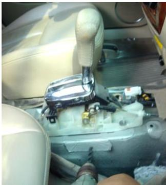
11. Drill a center hole of the bracket first. Please do not drill other two holes until adjust the lock in right position.
