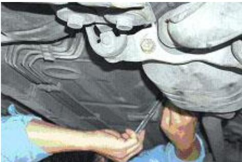
12. Uses the Screw 2 for the center hole of the bracket and screw it tight up with the wash 3 & wash 4. Then spray the Anti-Corrosive paint on the nuts to avoid gather rust.
