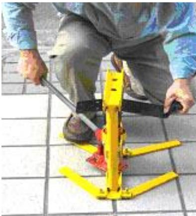
8. Band the bracket to suit the shape of gearbox with the banding machine, in order to screw the bracket tight on the metal board of the gearbox.
