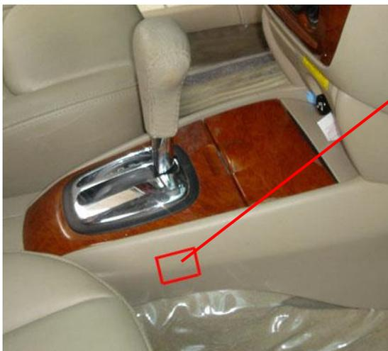
15. Cut off the square lock hole on the Plastic gearbox and put the gearbox back.
